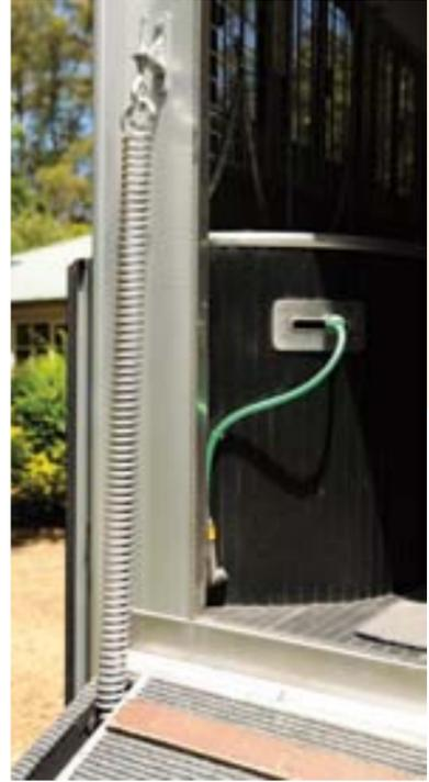
The springs provide an easy manual lift of the ramp. There are not always wash bays at competitions in New Zealand and the retractable hose hot wash is good for the horses and hosing out the horse section. There is an 800 litre water tank for all coach functions.
