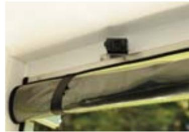
The closed circuit TV camera in the horse section and the roll down weatherproof cover for the back of the coach.
