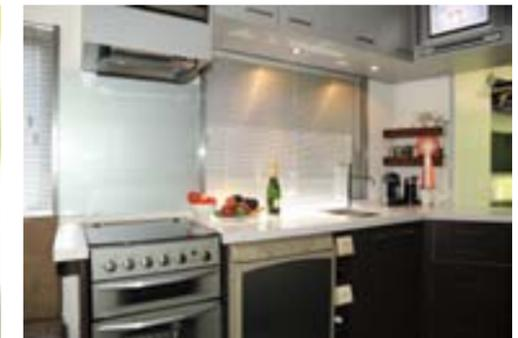
The kitchen showing the upright gas stove with separate pull out grill and the "three way" fridge. (Gas, mains power and 12 volt battery). The exhaust fan above the stove is ducted to the outside.
