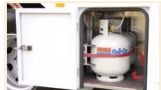
The gas supply (more efficient than electricity) powers the fridge, the oven/hob and hot water. The gas bottle has its own easy to access external box.
