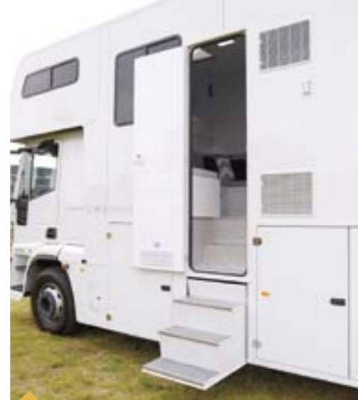
Both the steps and entry to the living area are manually operated. Electric steps and keyless entry are two of the little things that have not been included in this coach in an effort to keep the costs down. All these "little" extras add up.
