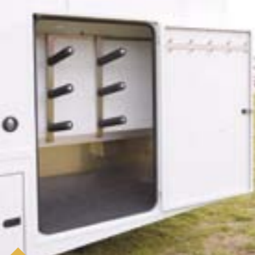
The external tack box carries six saddles. It is a Wade field trialled policy to have all the storage lockers on the exterior of the coach to avoid walking up and down the ramp all the time when tacking up.
