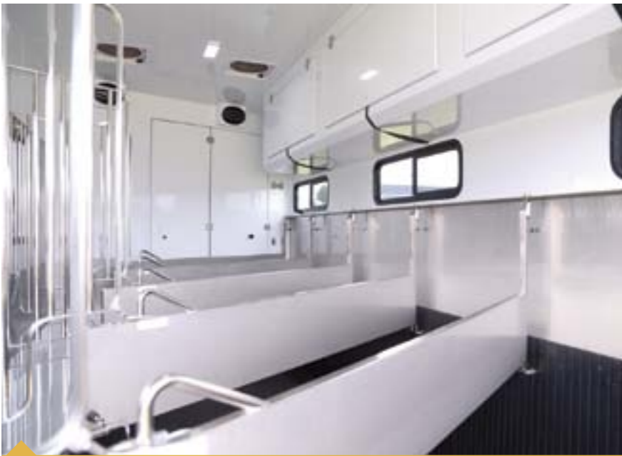
No chance of rust in this Coach. The stainless steel interior is easy to keep clean and the stainless steel behind the horses reduces the risk of friction and rubbing. The enclosed overhead rug compartments are completely dust free. The doors are on gas struts and the leads to aid opening and shutting are conveniently clipped up when travelling.
