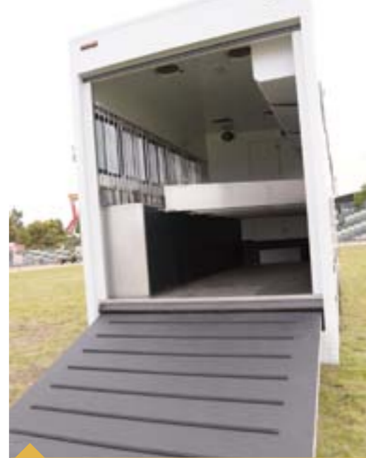
The ramp leading to the spacious and airy horse section. The ceilings are kept as high as possible to enable good air circulation. In a hot climate, horses always travel better with good airflow.
